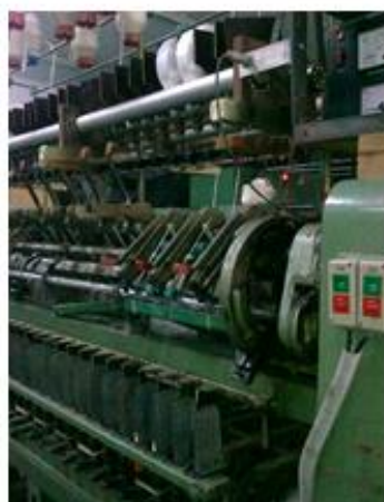
Production of Core-spun Yarn on simple ring frame spinning machine
